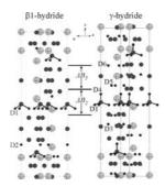
Hydrogenetion of ErNi<sub>3</sub> (rhombohedral PuNi<sub>3</sub> type structure) has been investigated by synchrotron and neutron powder diffraction. At least three hydride phases were found:  $\beta_1$ :  $x\sim1.3$ ;  $\beta_2$ :  $x\sim2$  and  $\gamma$ :  $x\sim3.7$ , the latter being stable only under hydrogen pressure (~100 bar). While the lattice expands mainly along c in the  $\beta$ -phases, it expands in the basal plane on transition to the  $\gamma$ -phases. In the  $\beta$ -
