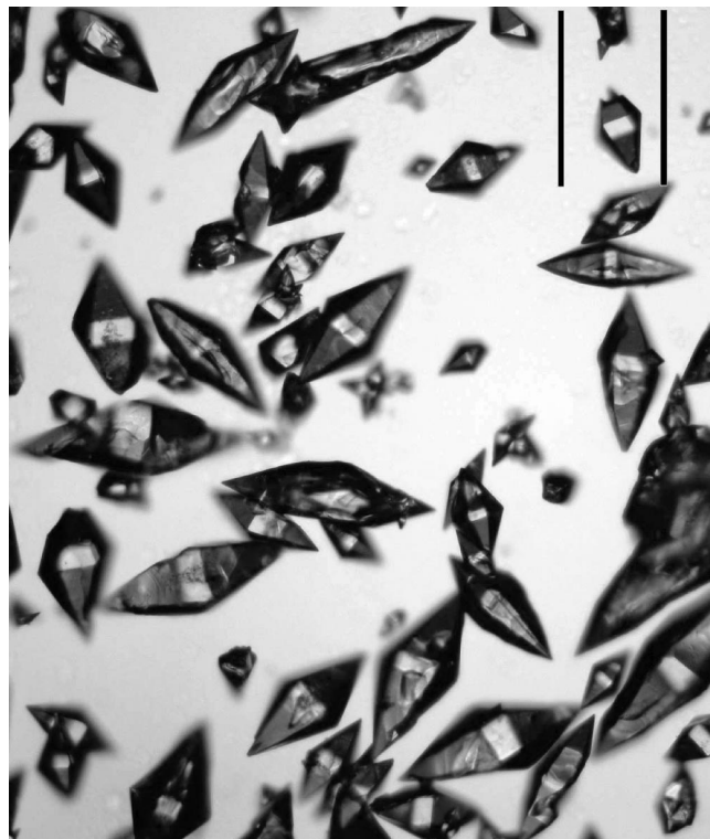
Figure 2. Single crystals of ScBDC prepared by the solvothermal method. Distance between the two black bars is 100 μm.
