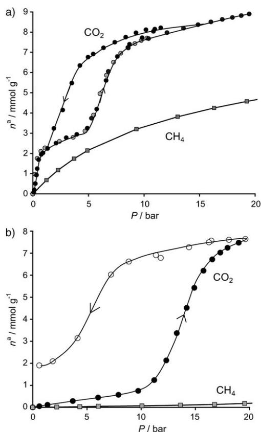
**Figure 2.** Comparison of the adsorption isotherms of carbon dioxide and methane at 304 K on a) dehydrated and b) hydrated forms of MIL-53(Cr). Grey- and black-filled circles represent two different experiments.  $n^a$  = amount adsorbed.
