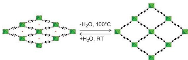
**Figure 1.** Hydration and dehydration process occurring in MIL-53(Cr, Al). Left: MIL-53LT (hydrated); right: MIL-53HT (dehydrated).
