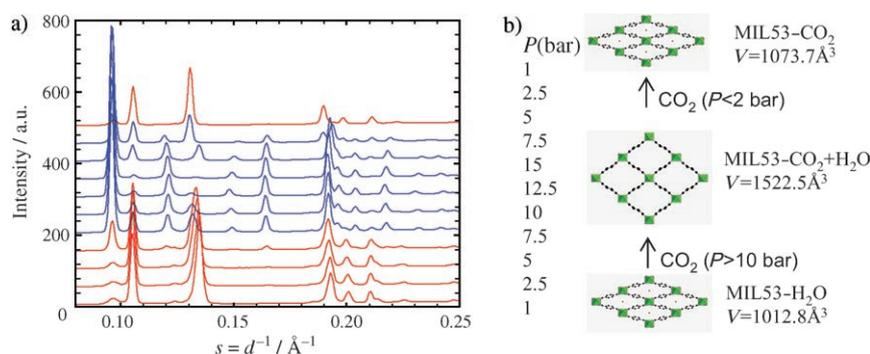
**Figure 3.** a) Evolution of X-ray diffraction patterns ( $\lambda = 0.71118 \text{ \AA}$ ) with increasing pressure of carbon dioxide for the hydrated MIL-53(Cr) solid. b) Schematic view of the resulting breathing phenomenon for MIL-53(Cr).
