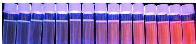
Fig. 2. Changes of the emission spectra at \lambda_{\text{ex}} = 500 nm (top) and UV light irradiated fluorescence color changes (bottom) of the solution of 1 (10 \mu\text{M} , \text{CH}_3\text{CN}-\text{H}_2\text{O} (9:1, v/v), 0.1 M HEPES buffer, pH 7.4) upon externally added hydrazine (0.01, 0.1, 1, 5, 10, 25, 50, 75, 100, 125, 150, 175, 200, 250 and 300 \mu\text{M} ). (For interpretation of the references to colour in this figure legend, the reader is referred to the web version of this article.)
