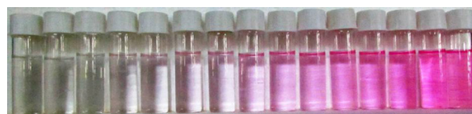
Fig. 3. Changes of the UV-vis spectra (top) and naked eye color changes (bottom) of the solution of 1 (10 \mu\text{M} , \text{CH}_3\text{CN}-\text{H}_2\text{O} (9:1, v/v), 0.1 M HEPES buffer, pH 7.4) upon externally added hydrazine (0.01, 0.1, 1, 5, 10, 25, 50, 75, 100, 125, 150, 175, 200, 250 and 300 \mu\text{M} ). (For interpretation of the references to colour in this figure legend, the reader is referred to the web version of this article.)
