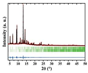
Fig. 8 Le Bail fit to the synchrotron radiation X-ray powder pattern  $(\lambda = 0.821693 \text{ Å})$  of the sample obtained by the reaction of 2-cyanopyrimidine with pyrimidine-2-carboximidamide. Experimental and calculated data are shown in red symbols and black line, respectively. Blue line shows the difference curve, while green marks show Bragg positions for  $\alpha$ -TPymT (top row) and  $\beta$ -TPymT (bottom row).
