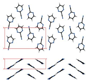
Fig. 4 Zigzag-like layers in the crystal packing of 2-cyanopyrimidine along the a (top) and b (bottom) axes.
