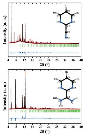
Fig. 3 Rietveld refinement plots ( $\lambda$  = 0.68884 Å) of 2-cyanopyrimidine (top) and pyrimidine-2-carboximidamide (bottom). Experimental and calculated data are shown in red symbols and black line, respectively. Blue line shows the difference curve, while green marks show Bragg positions. Insets show molecular structures of 2-cyanopyrimidine and pvrimidine-2-carboximidamide
