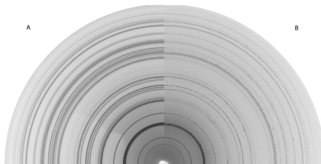
Figure 5. The two-dimensional diffraction patterns from a not fully crystallized sample (LidiSi-2) for the area exposed to the X-rays during the experiment (panel A) and the nonexposed area (panel B). The irregular radial intensity in panel B is typical for coarse grained samples.
